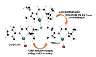
New copper(I) complexes of the guanidine-amine ligands TMGd<sup>i</sup>pae and DMEGd<sup>i</sup>pae were structurally characterised and theoretically investigated towards donor competition. The ligands proved to be useful in copper-mediated atom transfer radical polymerisation of styrene in bulk and MeCN solution.
