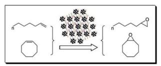
A series of supramolecular assemblies based on POMs modified by organic ligands were synthesized by a one-step hydrothermal method. They are active catalysts for the epoxidation of olefins
