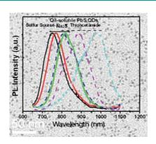
High-quality, oil-soluble PbS quantum dots (QDs) with tunable photoemission throughout the near-infrared (NIR) region (ca. 750–1000 nm) were synthesized by a two-phase approach, with use of water-soluble Na<sub>2</sub>S and thioacetamide, which differ in reactivity, as sulfur sources.
